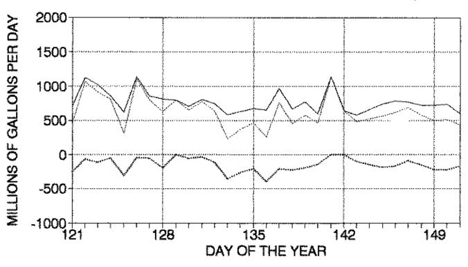
FLOW IN — FLOW OUT — NET FLOW OUT
